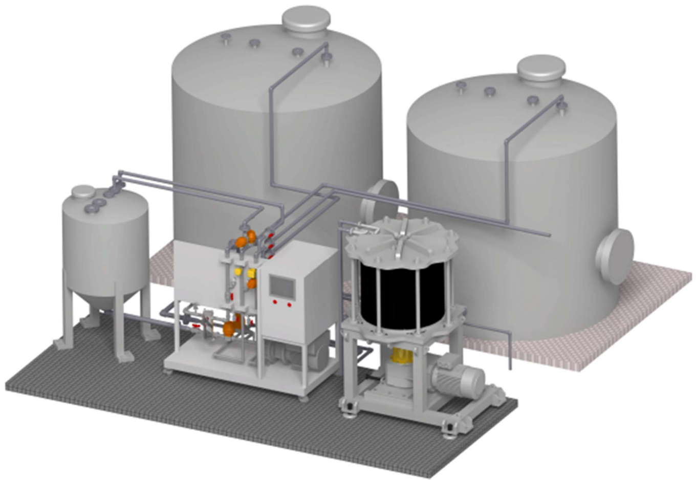
Figure 4: 3D layout of FMX-E5 pilot trailer (two auxiliary tanks are for reference and not included with the pilot trailer)
